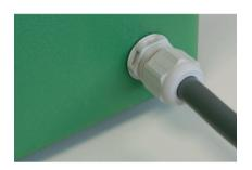
The supplied cable gland is suitable for a two-core cable with an outside diameter of 10 mm. Make sure the cable gland is sufficiently tightened. This also acts as a strain relief.
